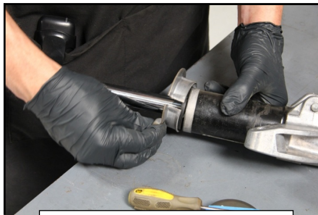
Photo 2: Removing Lower Spring Perch from Strut Body
