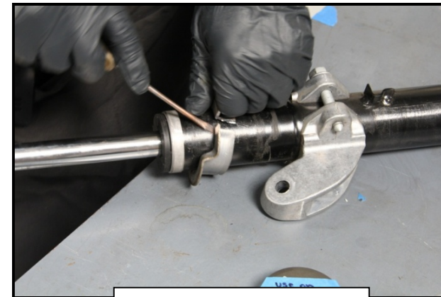
Photo 3: Prying Apart Lower Spring Perch
